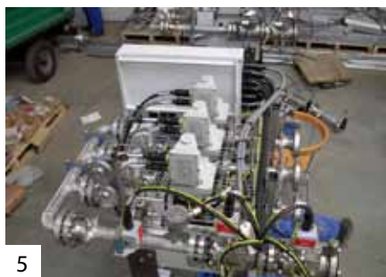
5 Mechanical and electrical detail design of a natural gas mixing station with a safety system for offshore gas turbine application.
