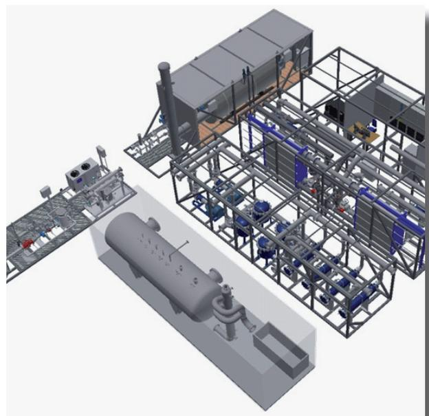
The MGTP (Mobile Geothermal Plant) is designed by GtS and built, based on many years of operational experience. It is a temporary geothermal installation consisting of six modules and can be deployed immediately after the production and injection wells have been drilled.
